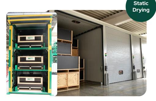
In **static drying**, seeds remain stationary while controlled relative humidity, airflow, and temperature gradually reduce their moisture content. This gentle drying process helps maintain seed quality by preventing overdrying and minimizing mechanical damage.
