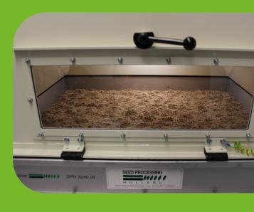
**Box drying** ensures controlled drying of various crops, including plant material and seeds, by dehumidifying process air, independent of ambient conditions. This preserves seed quality by achieving optimal storage moisture levels.
